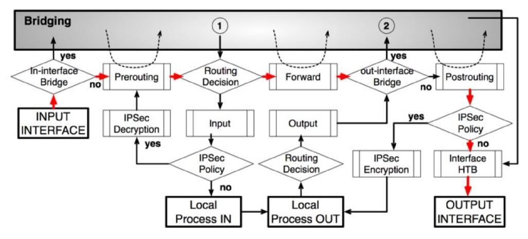
It Seems all packets flowing to / through the router are processed using the routing table
