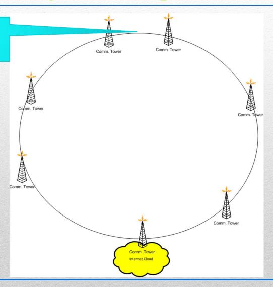
Traffic from tower to tower uses the most cost effective path.
