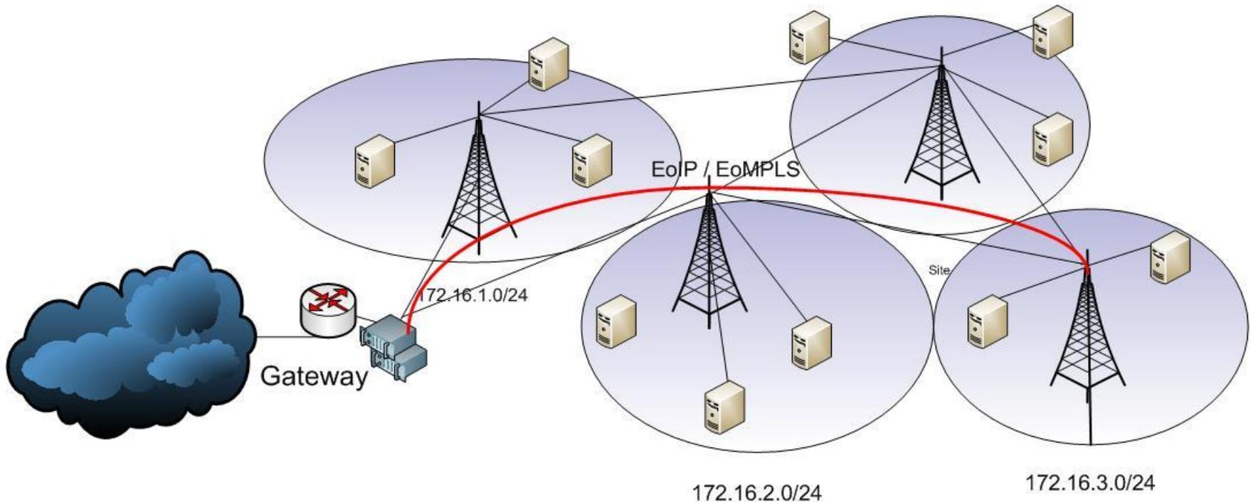
Usually dynamic routing with transparent tunneling from the customer to the main gateway – (EoIP / EoMPLS, etc)
