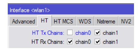
In order to use only chain1 the chain0 RX should be always enabled in order to make the wireless link to work
