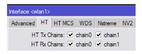
When board has both antennas connected it is suggested to use all the TX/RX chains to get the best speed and stability
