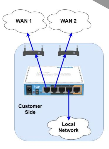
If the Internet Connection Unreachable, the MikroTik Router still can access the Gateway Modem, then it will never know the connection status, and the MikroTik Router still forward the packet to the modem
