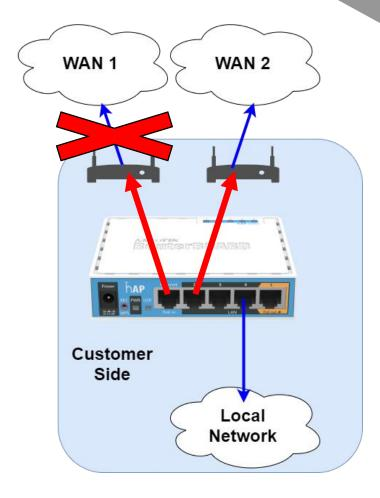
Using "/tool netwatch" to testing connection to an address outside the local network. Could be ISP Gateway or other Public Address.
