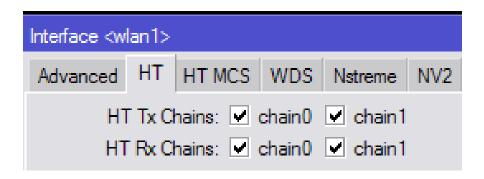
When board has both antennas connected it is suggested to use all the TX/RX chains to get the best speed and stability
