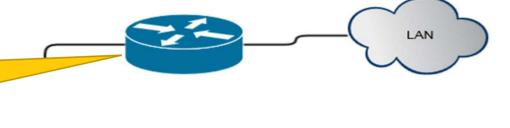
Underlying principle of rp\_filter is to block outbound traffic if the IP does not belong to the subnet that resides on the LAN
