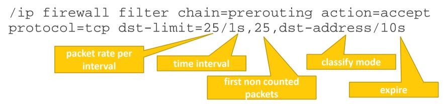
Match packets until a given pps limit is exceeded for every destination IP address and destination port combination.
