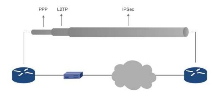
If PPP send from one site to other site, L2TP will encrypt to packet in L2TP Tunnel. And if we combine L2TP with IPsec, IPsec will encrypt L2TP Tunnel.
