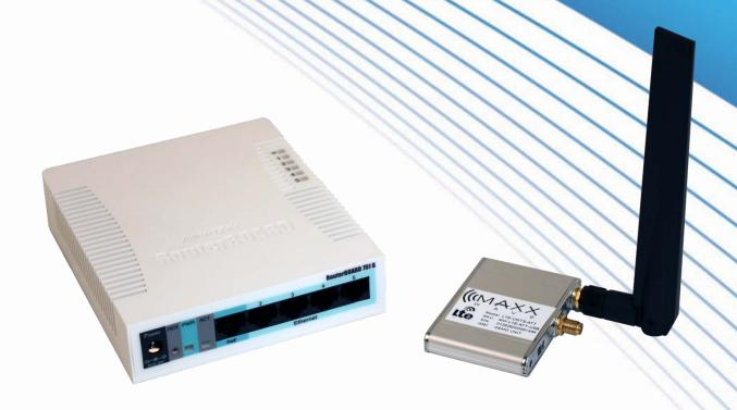
(RB/951G with USB Port and MaxxWave LTE USB Modem)
